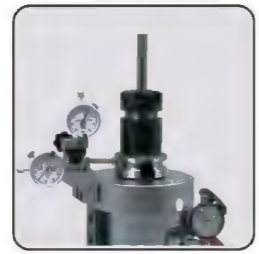
检测V槽位置和直径尺寸 verify the location and dimensional accuracy of the vee-flange
