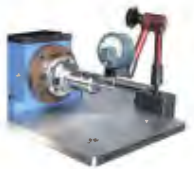
校正筒夹公差 Correction collet tolerances
