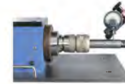
校正刀杆公差 Correction shank tolerances
